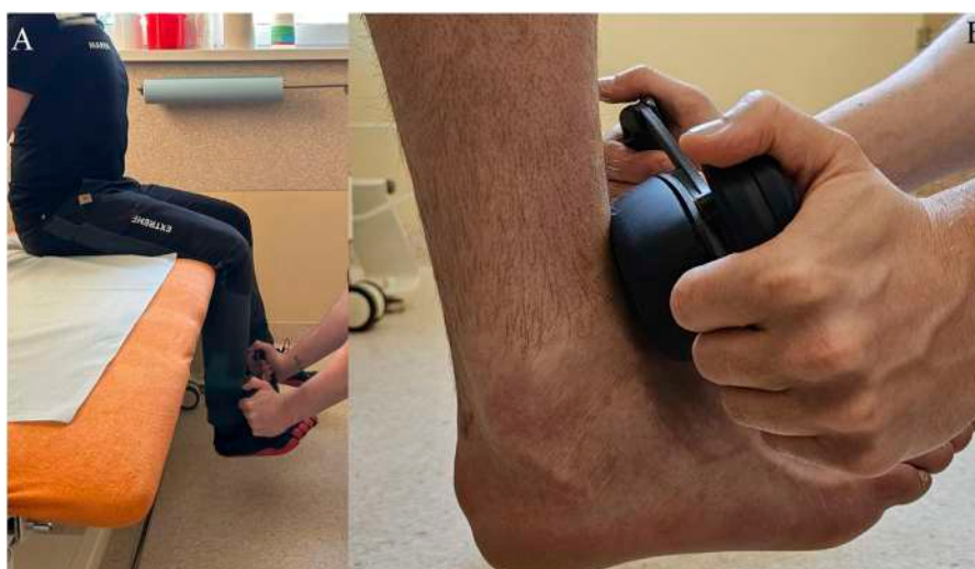
FIGURE 1 Test position of the Kinvent K-Push handheld dynamometer during testing procedure (A) and the measurement point (B).
