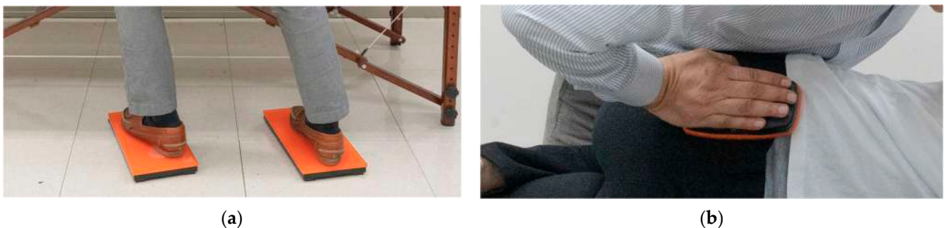
Figure 1. (a) Force plate between the experimenter's feet and the ground; (b) Muscle controller (load cell) between the experimenter's hand and the surface in contact with the skin.
